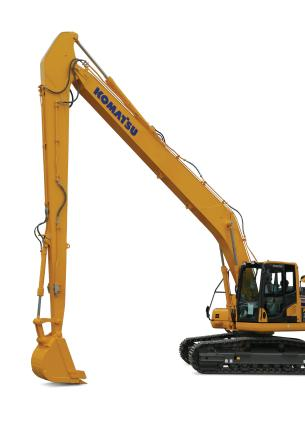
Easy switching between long reach attachment and standard attachment
